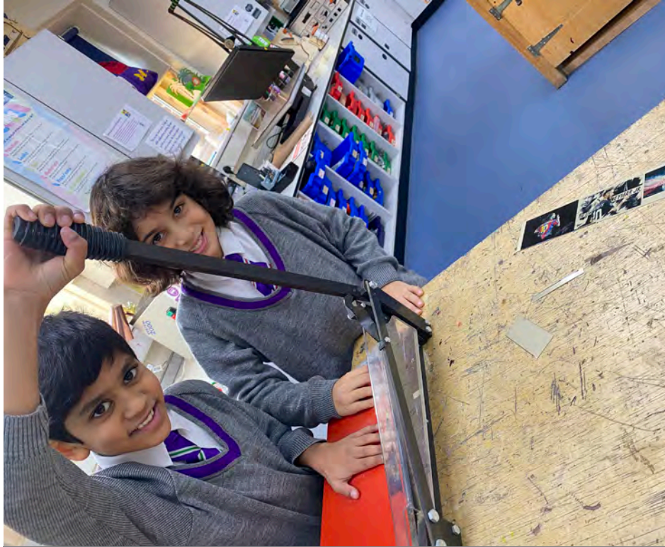
Noah and Arjan using the guillotine to cut sheet aluminium.
